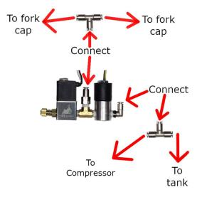
Connect the fill and dump valve wires to the Front Air Add-on Module per the below diagram.
