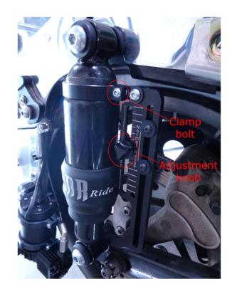
4. Wire the limit switch per the included wiring instructions, ensuring that there is enough slack for the adjustment knob's full range of adjustment.
