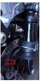
3. Once the shock is installed, ensure the entire RHR assembly clears its surroundings. Then tighten the clamp bolt to secure the top of the RHR to the shock.
