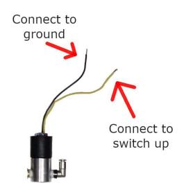
4. Wire the dump valve, connecting the white wire to the "Down" switch, and the black wire to ground.
