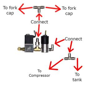
3. Wire the fill valve (using the provide blade terminals if needed), connecting the yellow wire to the "Up" switch, and the black wire to ground.
