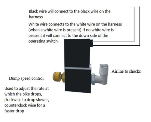
Mounting is at the discretion of the installer. We typically mount with double sided tape to the ABS in a way that the speed control is accessible
