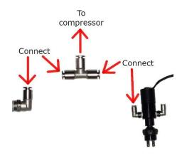
3. Connect the other side of the fill valve (side engraved "S") to the other provided tee and connect the tee to the shocks.
