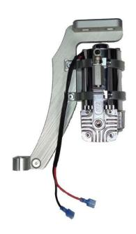
2. Remove the two bolts from the rear of the saddlebag mount rail. Install the Boom 2 compressor mount onto the bag rail, using the provided bolts and the factory nuts.
