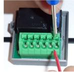
b. Insert the wire so that the exposed wire is as far towards the back of the terminal as possible. Ensure that the end of the wire coating is past the outer edge of the terminal. This will reduce the risk of the wires wiggling loose and prevent short circuits.
